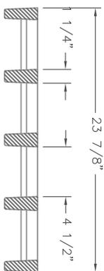
NOTE: FRAMES ARE FURNISHED IN STANDARD 2'-0" INCREMENTS. GRATES ARE FURNISHED IN STANDARD 2'-0" INCREMENTS. SPECIAL LENGTH GRATES CAN BE FURNISHED FOR ANY OVERALL LENGTH. EACH GRATE HAS A FREE OPEN AREA OF 1.04 SQUARE FEET.
